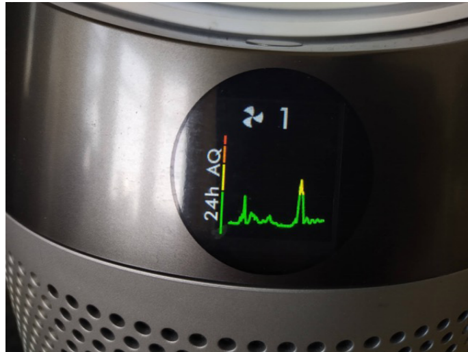
Example of an IAQ monitor. Monitoring in real time is useful but monitoring over a period of time is more beneficial so trends can be found
