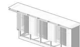
Vertical Solar Protection Glazed openings screened by angled vertical louvers to diffuse daylight into the building. The open wood work reacts to the building's structure, altering it gently.
