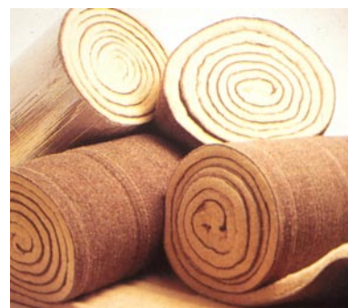
This natural wool product is biodegradable, healthy and as good as mineral wool for insulation. Source: F. Stevenson
